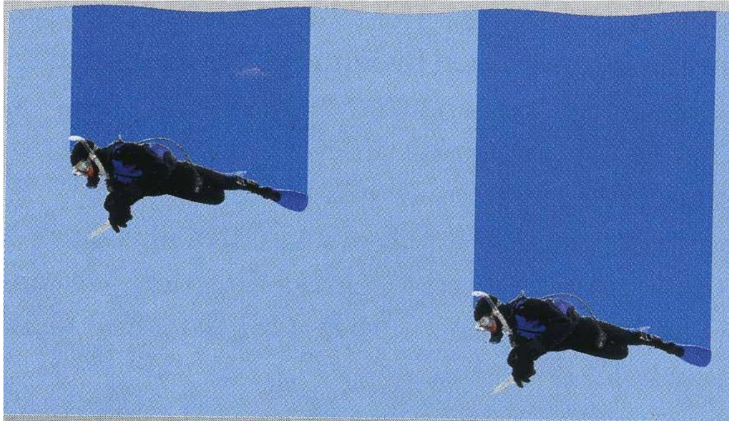
Diagram 6.4 Diver at two different depths in water showing columns of water resting on her
